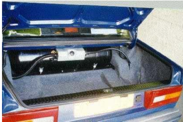
Figure 2. Typical Conversion of Vehicle to LPG
