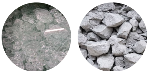
Demolished glass and concrete from LMA
