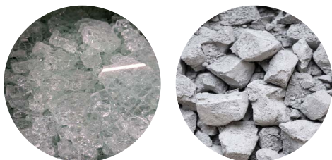
Demolished glass and concrete from LMA
