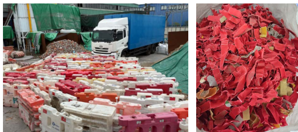
Water Barriers Shredded
